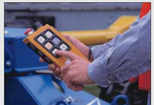
Radio remote control operation
