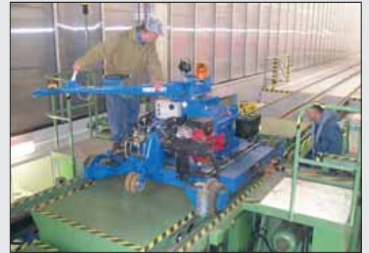
Operation on underfloor lathe
