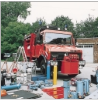
Rescue vehicle ZW 82 S with rerailling equipment and front hydraulics.
