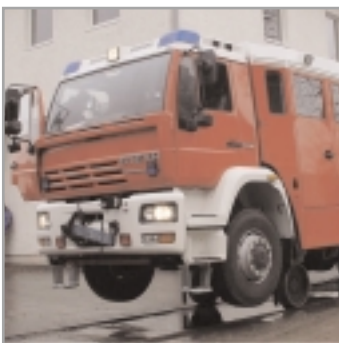
Loctrac ZW 202 S with hydrostatic drive.
