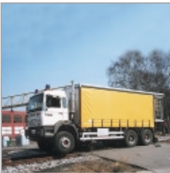
ZW 102 S fire fighting truck with track guiding system.
