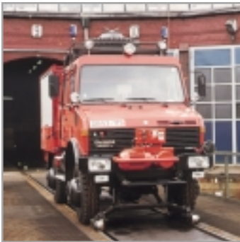
Rescue vehicle ZW 100 S with double cabin for 7 persons: Auxiliary unit for derailed wagons. Operating at Federal German Railways DBAG.
