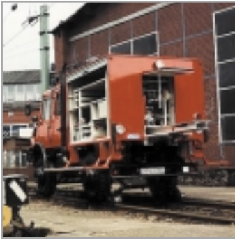
Rescue vehicle ZW 100 S: rear view with retractable floors for loading rerailling equipment.
