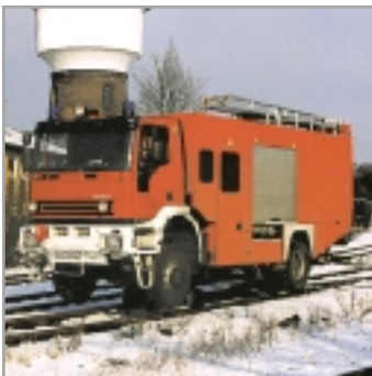
Loctrac ZW 202 S with hydrostatic drive.
