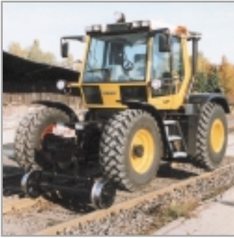
ZWEIWEG track guiding device with friction drive.
