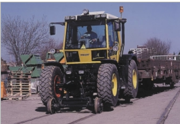
Fendt tractor approved for operating on tracks of German Railways DB AG.
